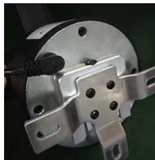
Hang the device to the holder, lock with screw, now the device is ready to setup to Cloud.
