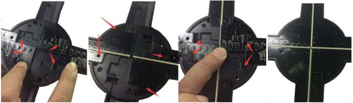
Lock the screw after LED board inserted to the base, pay attention 8 longer screw and 4 shorter screw for different position as below (red arrow for shorter TM4x5, Blue arrow for TM4x8):
